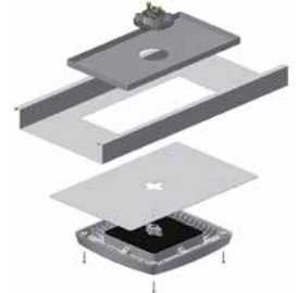
Rectangular Hole Kit (678291WHT) Includes cover panel, top plate, hardware and sealant
